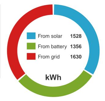
The property is expected to consume 4500kWh of electricity each year. Around 34% of this (1528 kWh) is expected to be supplied directly by the solar array. Another 30% (1356 kWh) is supplied from the storage battery. The remaining 36% (1630 kWh) is supplied from the grid.
