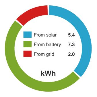
This graph shows modelled consumption data over the course of the selected day (March 27th). Total electricity consumption on this day was 14.6 kWh, of which 5.4 kWh (37%) is expected to be supplied directly by the solar array, and a further 7.3 kWh (50%) drawn from the battery storage system. The remaining 2 kWh (14%) is imported from the grid.
