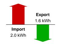
This graph shows the modelled import and export of electricity over a selected day (March 27th). On this day 2.00 kWh is expected to be imported from the grid, and 1.6 kWh exported.At times when no import or export is shown the battery storage system is charging or discharging.
