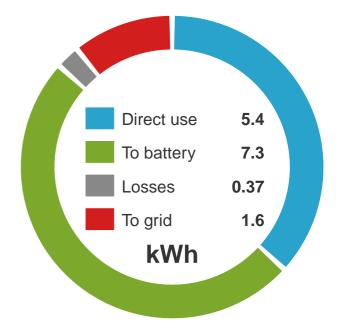
This graph shows the modelled profile of electricity generated by the PV array on a selected day (March 27th). On this day the PV system is expected to generate 14.6 kWh. Of this, 5.4 kWh (37%) is used directly in the property, 7.6 kWh (52%) is stored in the battery for later re-use, and 1.6 kWh (11%) is exported to the grid.
